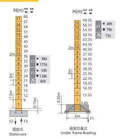
独立高度最大臂长的自重 (不含平衡重,不含压重) Weight with max free standing, max jib (without counter-jib ballast and load)
