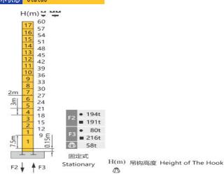
●工作状态反力 Reactions in service ■ 非工作状态反力 Reactions out of service 独立高度最大臂长的自重(不含平衡重,压重) Weight with max free standing,max jib(without counter-jib ballast and load)
